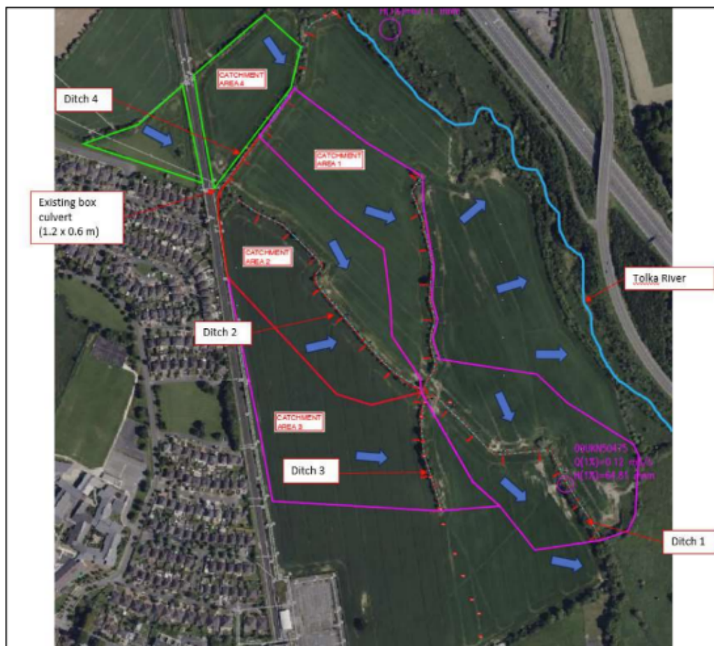
Figure 8.4 Existing drainage ditches across the Site and surrounding lands (source: ESR (DBFL, 2024))
